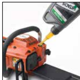
Special cap on 1 Litre can to prevent spillage
